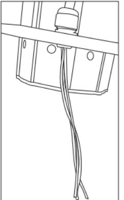
The phases of heaters 1 + 2 are connected to phase 2, black of the spiral cable using a connection terminal (3-pin) and the phases of heaters 3 + 4 are connected to phase 3, grey using a connection terminal (3-pin).
