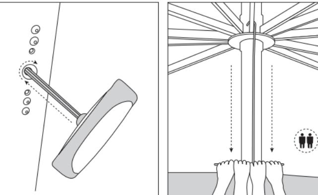
**Recommissioning after emergency closing:** With the motor drive disconnected, press the «Close sunshade» button and wait until the motor stops automatically once the sunshade is in end position. Completely close the sunshade by hand. Insert the Allen wrench into the opening at the pole by 6 mm and turn it in a counter-clockwise direction by approx. half a rotation. Remove the Allen wrench. Press the «Open sunshade» button to check functionality.
